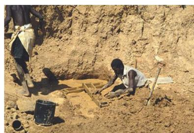
Figure 2: Slopmaking in a triple mould, Zimbabwe. ©Practical Action/Theo Schilderman
